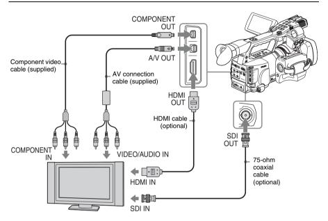
Regardless of whether the signal is HD or SD, the same status information and menus can be displayed on the external monitor as those on the LCD monitor/EVF screen.
